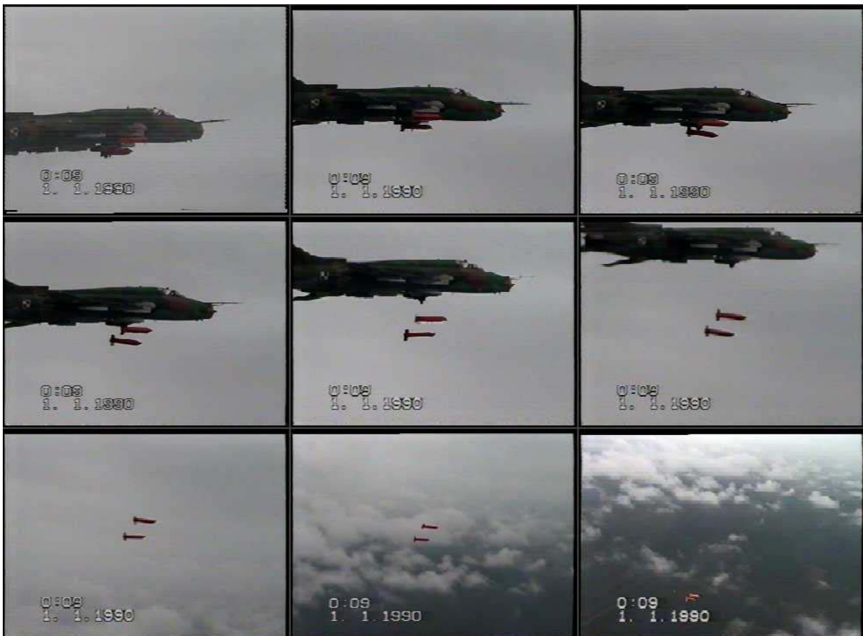
Figure 21: Frame photos of airdrop (high-speed camera on following aircraft)
