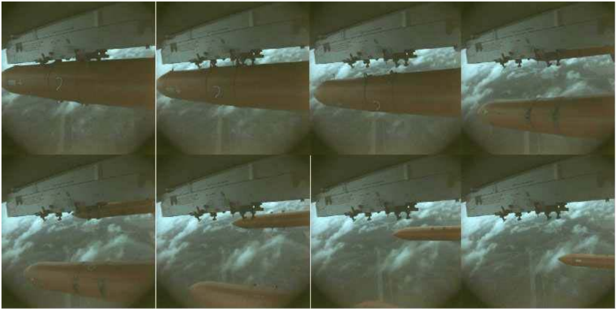
Figure 20: Frame photos of airdrop (on-board high-speed camera)
